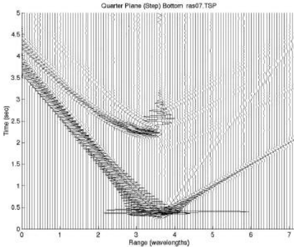
Figure 10b. An Example of plotting only the traces in the bottom set of receivers in the TSP file.
